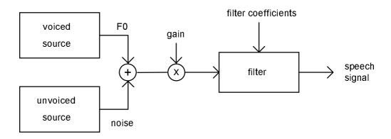
Fig. 1.2. Source-filter model of speech.
