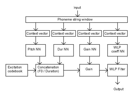
Fig. 5.8. An example of using neural networks in WLP synthesis (Karjalainen et al. 1998).
