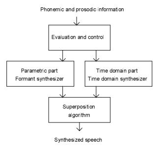
Fig. 5.7. Basic idea of the hybrid synthesis system
