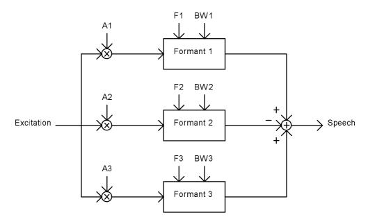
Fig. 5.2. Basic structure of a parallel formant synthesizer.
