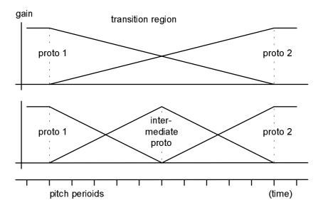
Fig. 5.5. Linear amplitude based interpolation (Lukaszewicz et al. 1997).
