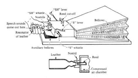
Fig. 2.2. Wheatstone's reconstruction of von Kempelen's speaking machine (Flanagan 1972).
