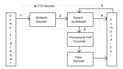
Fig. 7.1. MPEG-4 Audio TTS decoder architecture.
