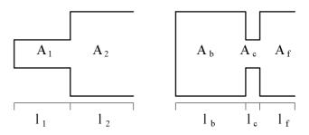
Fig. 3.6. Examples of two- and three-tube models for the vocal tract.
