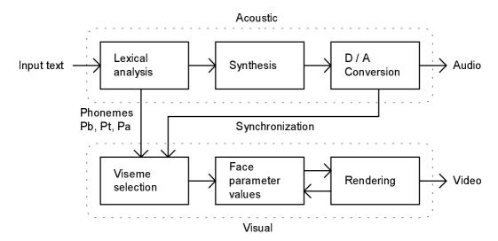
Fig. 8.1. Structure of the audiovisual synthesizer.
