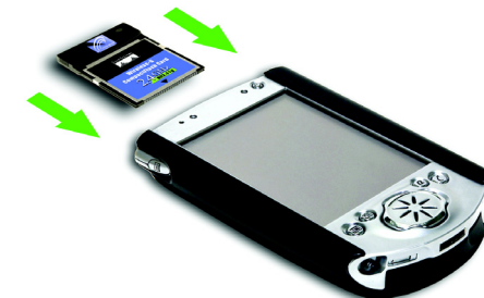
Figure 4-2: CompactFlash Installation into PDA
