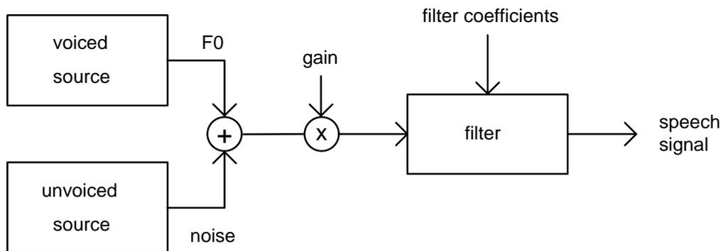
Fig. 1.2. Source-filter model of speech.
