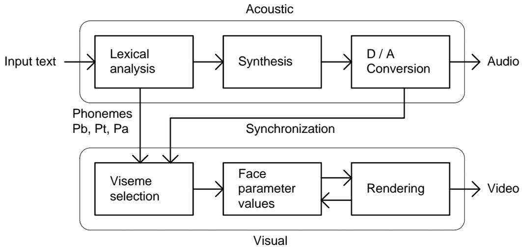
Fig. 8.1. Structure of the audiovisual synthesizer.
