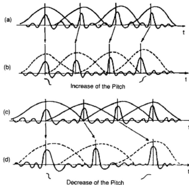
Fig. 5.4. Pitch modification of a voiced speech segment.
