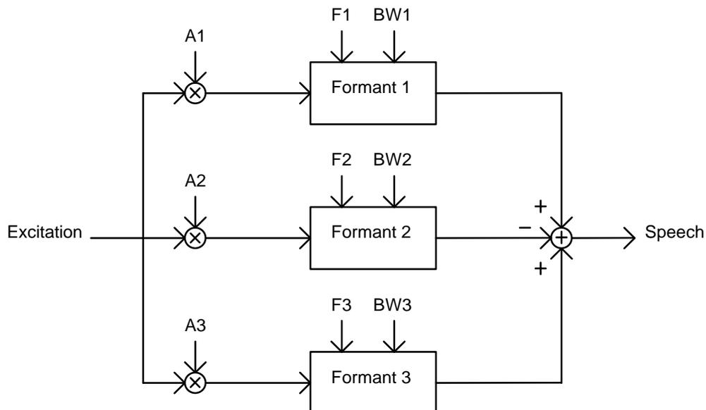
Fig. 5.2. Basic structure of a parallel formant synthesizer.
