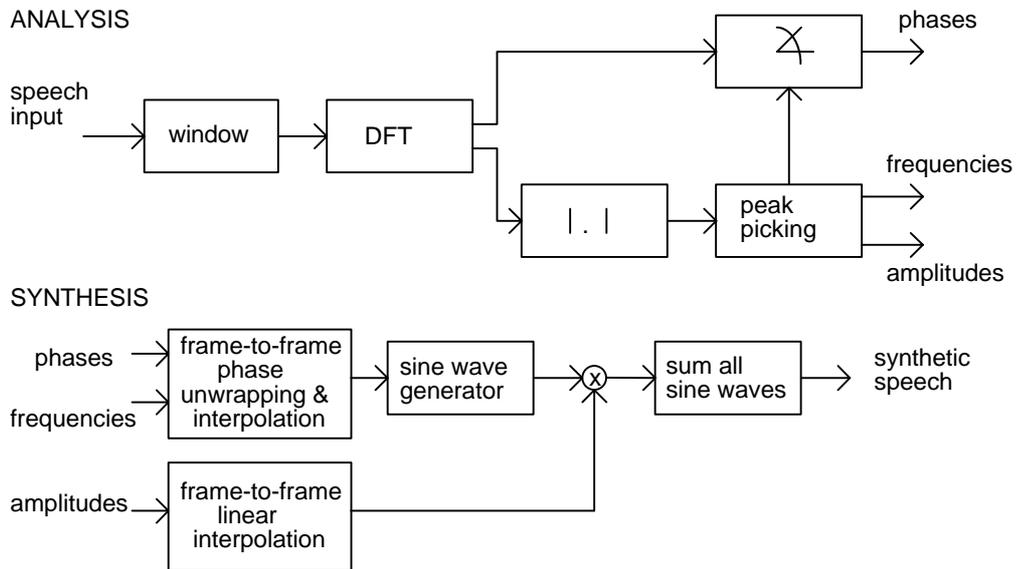
Fig. 5.6. Sinusoidal analysis / synthesis system (Macon 1996).
