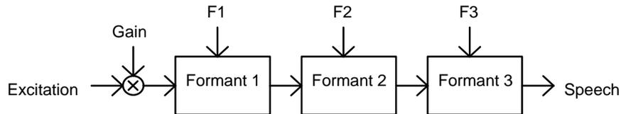
Fig. 5.1. Basic structure of cascade formant synthesizer.
