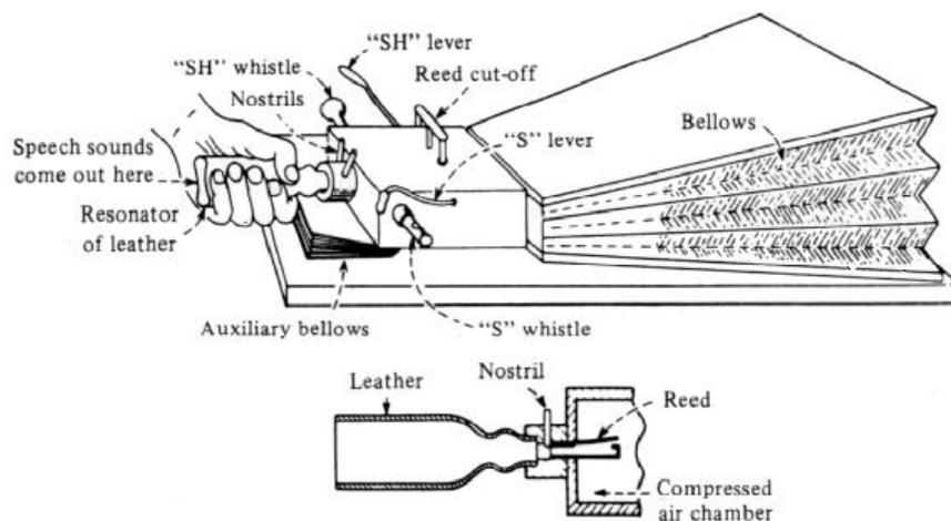
Fig. 2.2. Wheatstone's reconstruction of von Kempelen's speaking machine (Flanagan 1972).
