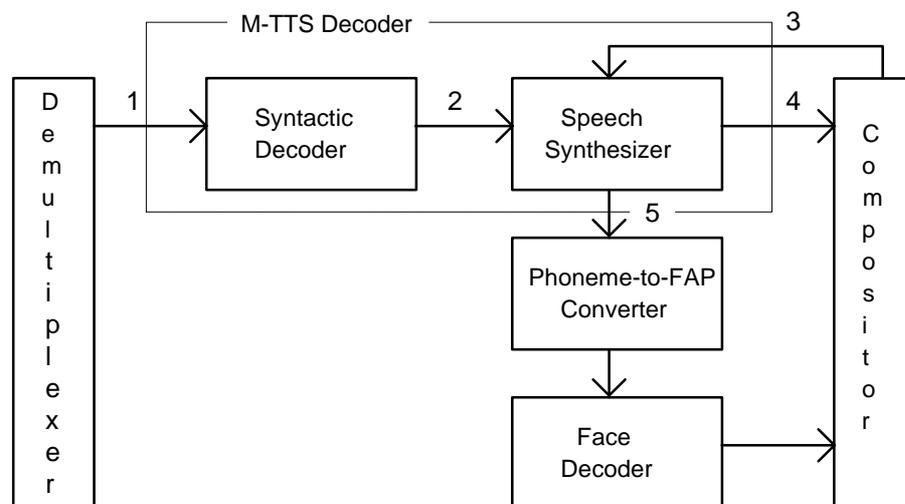
Fig. 7.1. MPEG-4 Audio TTS decoder architecture.
